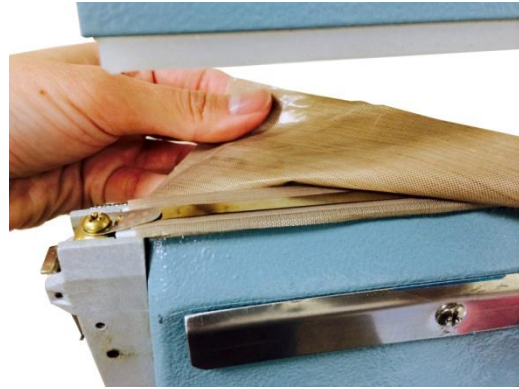
Figure 8. Pull PTFE cover to expose heating element.
