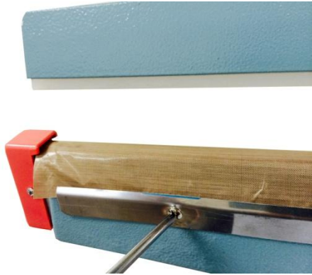
Figure 7. Loosen screws on PTFE plate.
