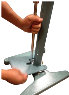
Figure 6. Attach pulling pole to the foot pedal.
