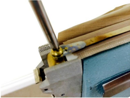
Figure 9. Screw element in place
